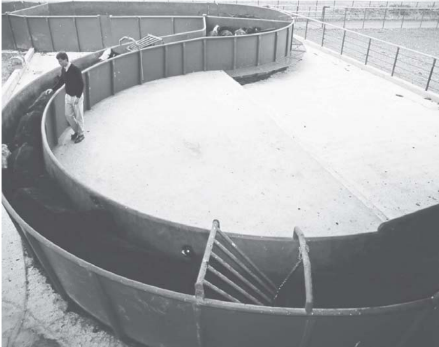
Curved chutes work better than straight ones (in which animals may turn back in the direction they came from). Note the two back-stops which hinge up as the animal passes under them.
