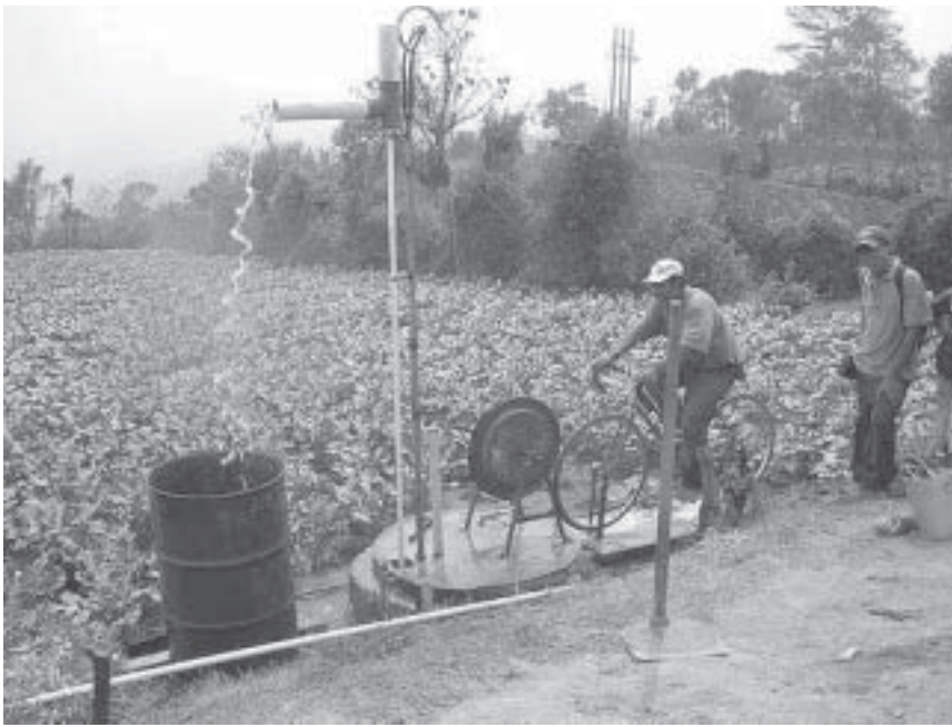
A bicycle-powered water pump in Guatemala.
